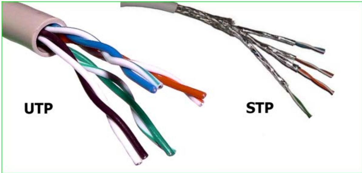
There are different ways to shield an Ethernet cable, but typically it involves putting a shield around each pair of wire in the cable. This protects the pairs from crosstalk internally. Manufacturers can further protect cables from alien crosstalk by screening UTP or STP cables. Technically the picture above shows a Screened STP cable (S/STP).
